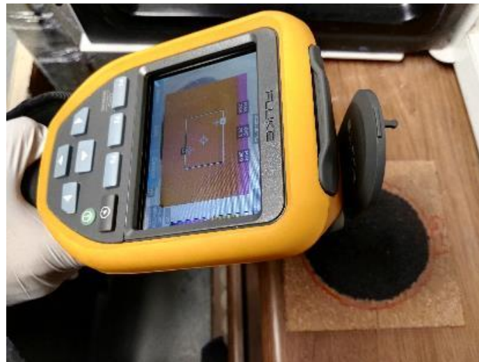
Figure 16. Infrared thermal imager to measure the temperature before and after microwave irradiation.
