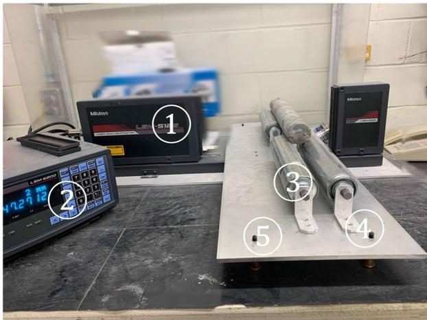
Fig. 5 Apparatus of rock core diameter measurement with rock sample
