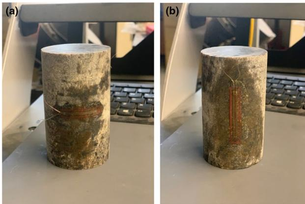
**Fig. 8** Sample instrumentation: **a** Horizontal strain gauge; **b** Vertical strain gauge
