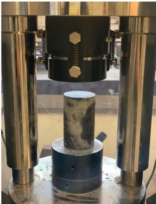
**Fig. 9** Setup of UCS test
