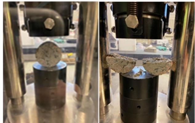
**Fig. 3** Brazilian test set-up on a Stanstead granite core
